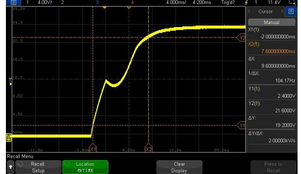
INPUT=230VAC/50HZ @ FULL LOAD CH1: Output Voltage
